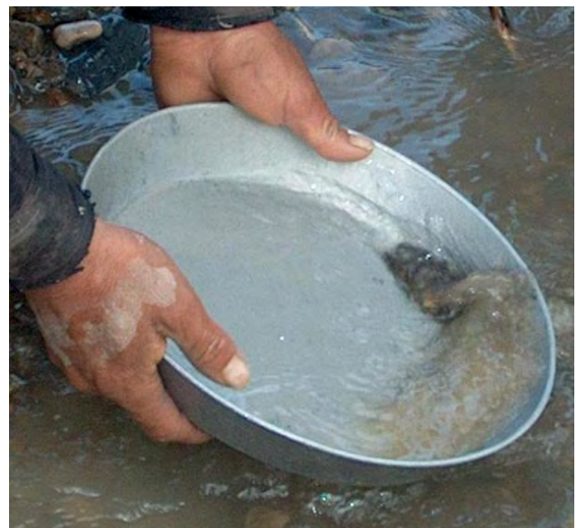
Figure 3. Panning in the same manner as for the North American Gold Pan. Kyrgyzstan. (photo: Robin Grayson)
