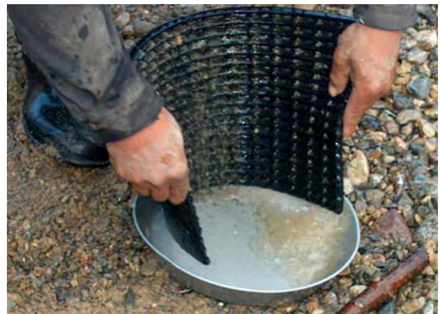
Figure 2. Artisanal miner loading concentrate from the ribbed rubber mat into an aluminium pan. Kyrgyzstan. (photo: Robin Grayson)
